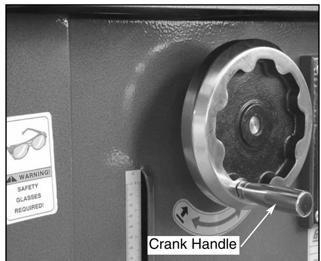
Figure 5. Handwheel mounted to shaper.
